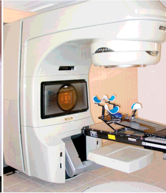
Figure 9 Portal Vision electronic portal imaging system with robotic support arm.
