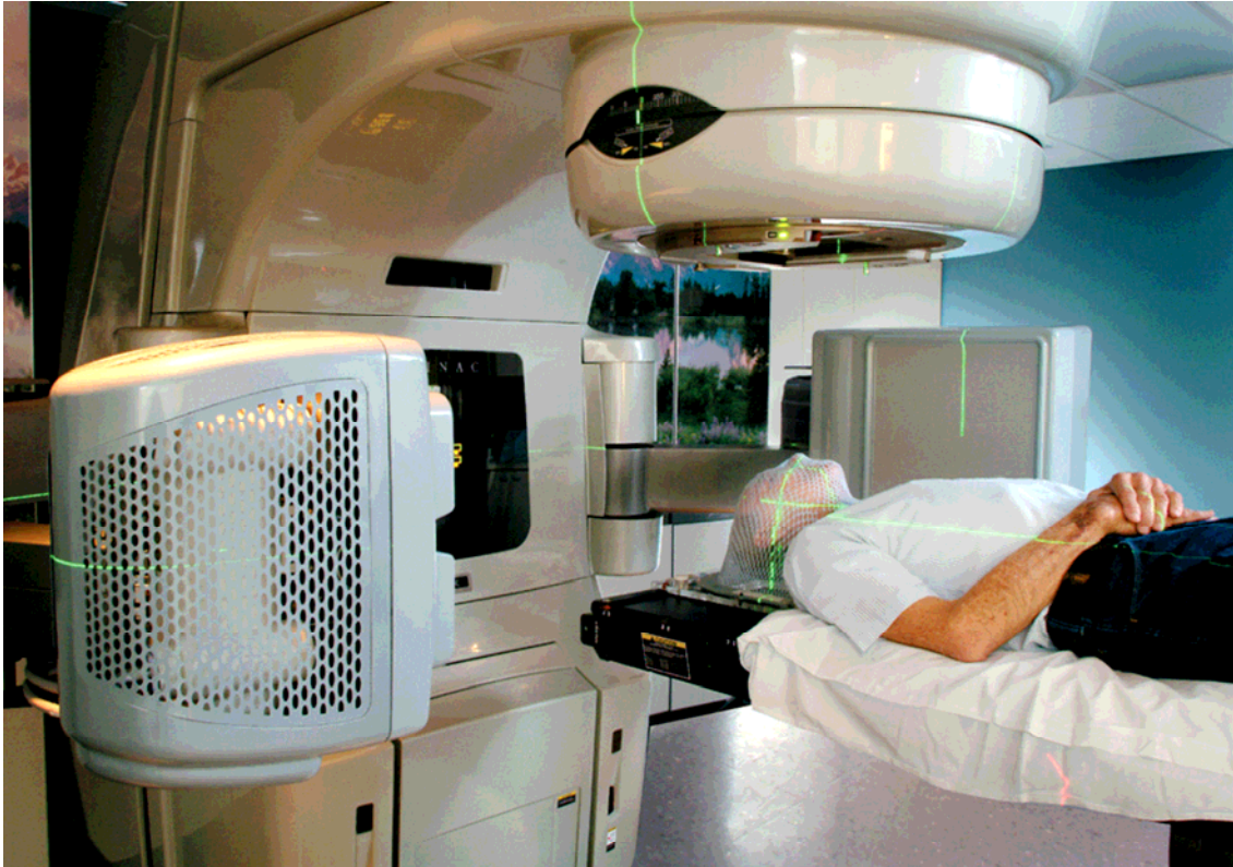
Figure 10: Clinac with On Board Imager. The system incorporates of an X-ray tube and an amorphous-silicon flat-panel image detector on a pair of robotic arms. (Image courtesy Emory University, Atlanta, Georgia, USA).
