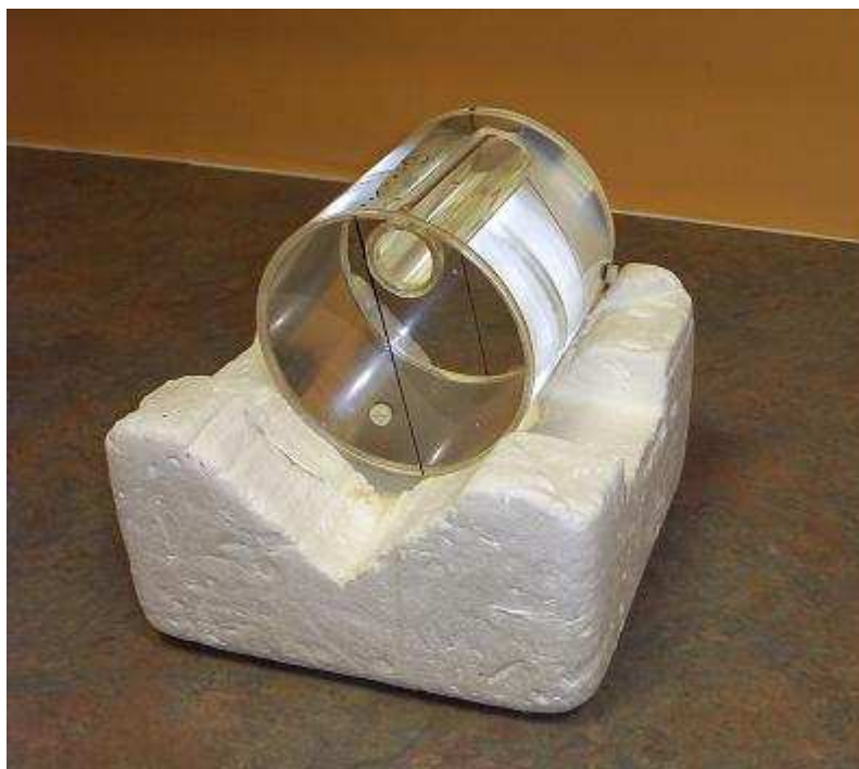
Fig 6.1.1 Neck phantom used in syringe ^{131}\text{I} calibrations
